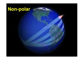
Satellite is ~36,000 km above earth the equator. Same rotation period as earth's. Appears 'fixed' in space. Circular orbit constantly moving relative to the Earth at 160-2000 km. Can be in Polar or non-polar orbit
