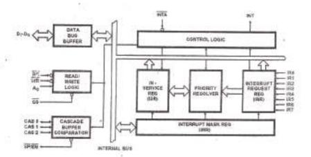
The architecture of 8259 can be divided into the following parts:
