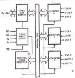
The architecture of 8254 can be divided into the following parts:
