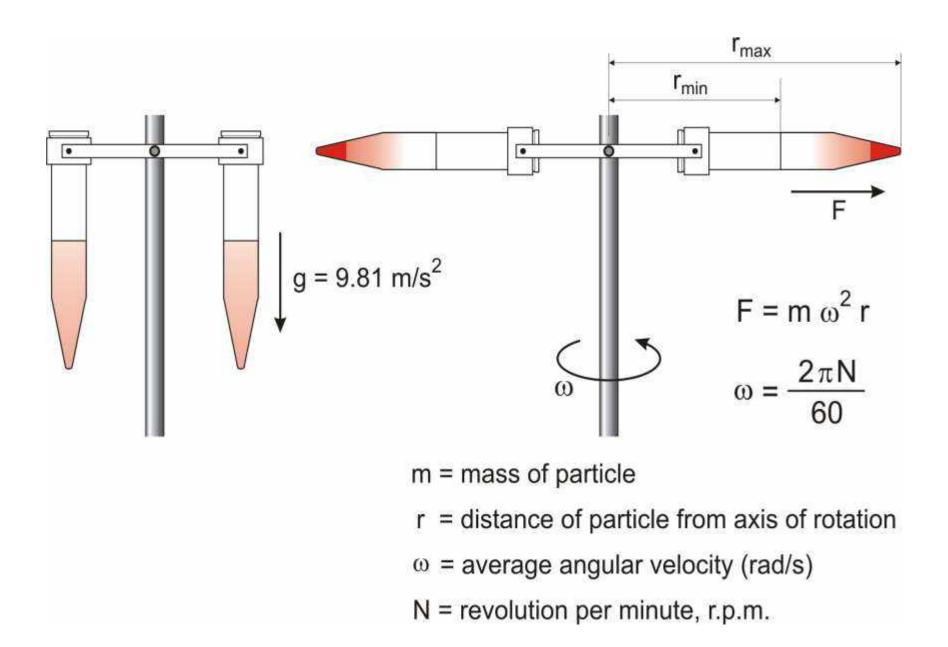
**Centrifugal force:-** The tube containing the suspension of particles is rotated at a high speed, which exerts a centrifugal force directed from the center of the rotor towards the bottom of the tube.
