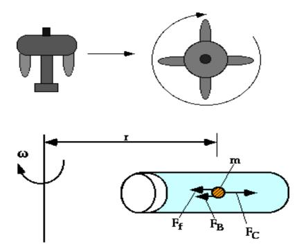
The particle (m) is acted on by three forces: FC: the centrifugal force FB: the buoyant force Ff: the frictional force between the particle and the liquid
