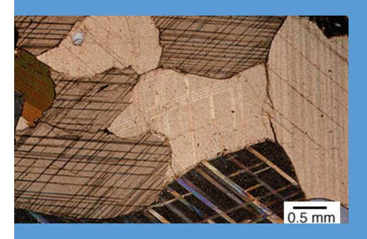
• The mineral calcite can be easily twinned during deformation, producing polysynthetic twins
