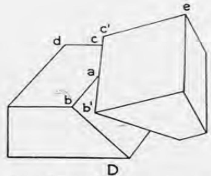
**Slip:** the relative displacement of formerly adjacent points on opposite side of the fault , and it is measured in fault plane .
