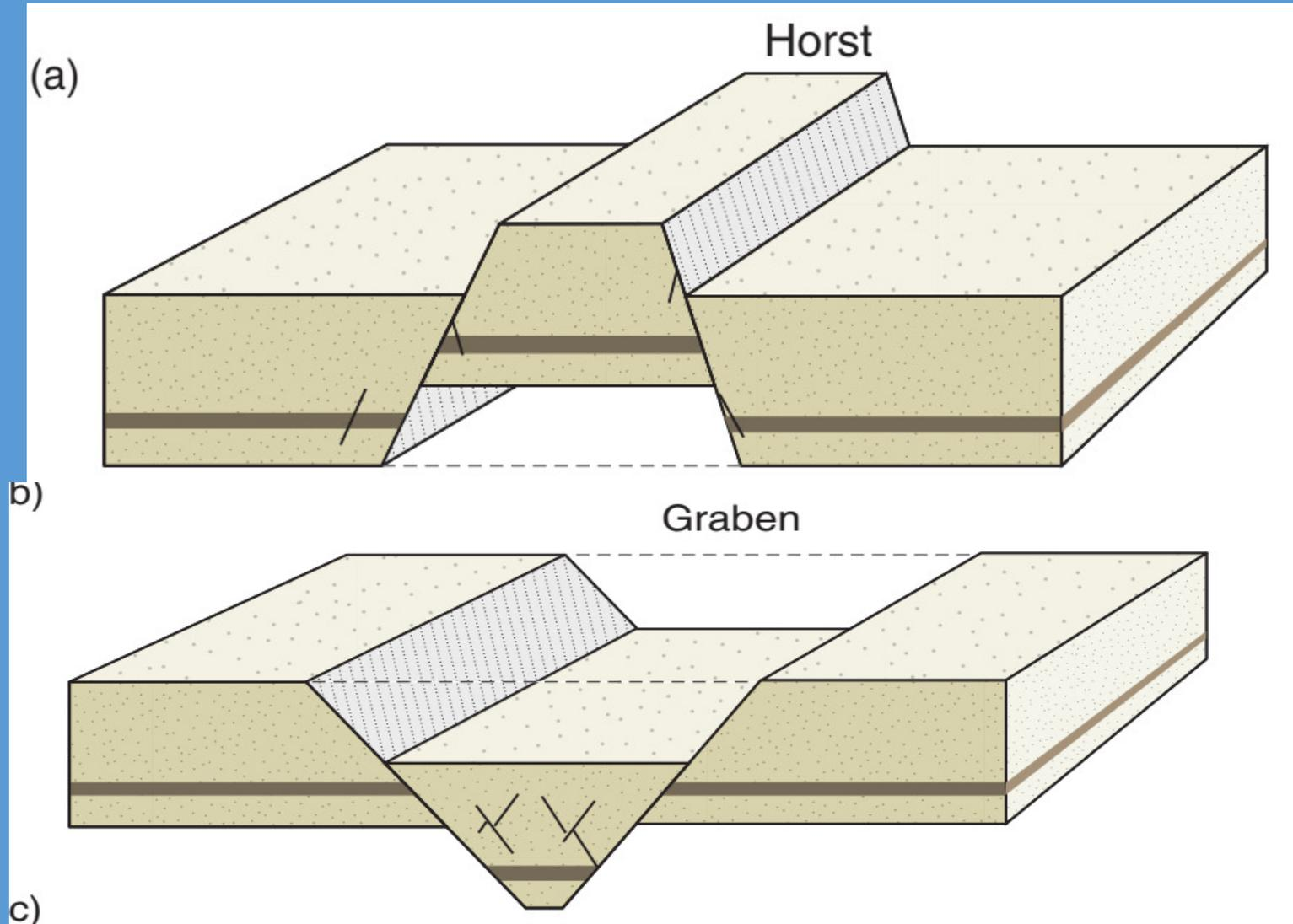
The two separations recorded in a vertical section are more commonly referred to as **heave** (horizontal component) and **throw** (vertical component)
