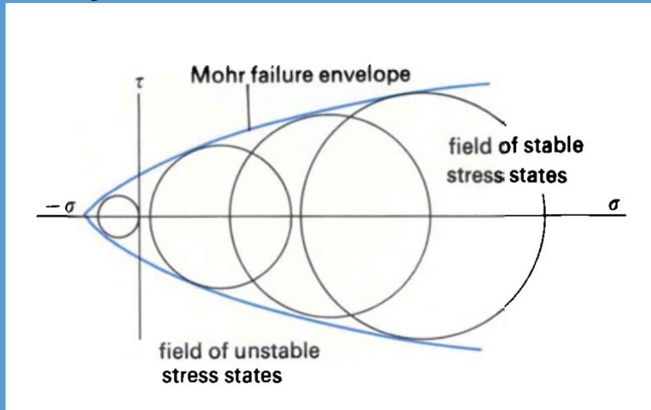
The Mohr failure envelope joining points of failure for different stress states separates the field of stable stress states from the failure field. Note that the shape of the Mohr curve implies an increase in the values of the shear stress  $\tau$  and fracture angle  $\theta$  with an increase in the mean stress.
